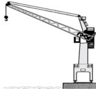
CODE C47 Wharf Side Crane: (Railmounted)
